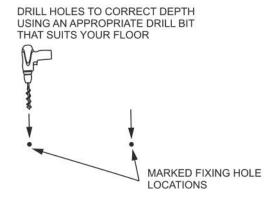
4. The floor plug should be inserted into the hole, then place the pan into position. Install the floor fixing kit as shown below. Take care not to damage the pan.
